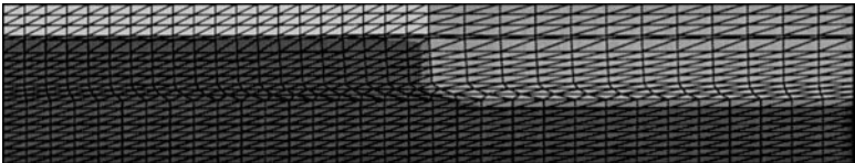
FIG. 24. Materials at the end of annealing following filling of the trench: the nitride mask (light gray region at the top left), silicon substrate (bottom dark gray region), deposited oxide (light gray region at top right), and thermally-grown oxide (light gray region separating the silicon substrate from nitride mask and deposited oxide).
